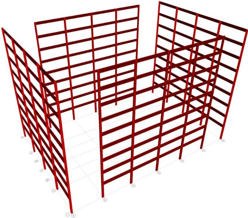
Figure 4: 3D rendering of archetype lateral frames only
